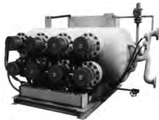
STEAM SUPERHEATER 600V 324KW 150 PSIG OPERATING TEMP. 750°F
